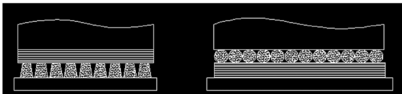
Figure 2. Two sides of a foundation constructed on layers of timber in many traditional buildings shown in Figure 1 (Masooleh, north of Iran).
