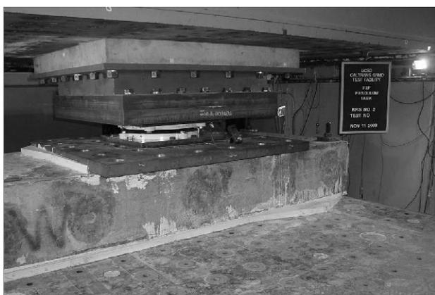
Figure 6. Isolation unit being tested at the SRMD Laboratory in San Diego (CA, USA).
