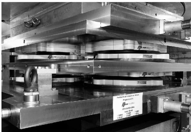
Figure 16. Six isolation units being tested at the FIP Industriale Laboratory.
